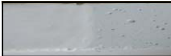
WAM® HTC SA, applied to castable by brush and sanded smooth after air drying, compared to mold surface.
